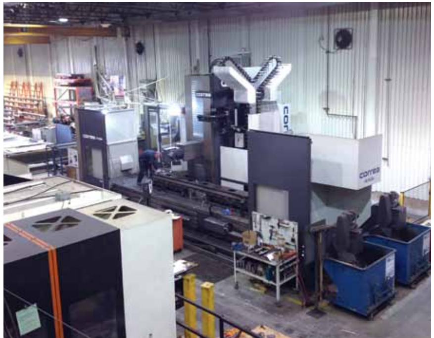
OSI Précision’s most recent investment, a six axis Axia-70 machining centre from machine builder Correa (purchased from Elliott Matsuura Canada) has helped the company reduce setup times and bring in new types of work.
