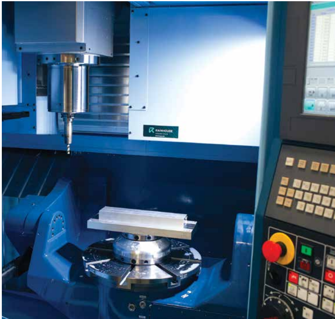
The Matsuura five axis machine has reduced setup times and increased throughput and efficiency at Rainhouse Manufacturing Canada.
